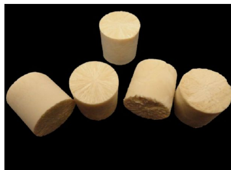
Figure 1. Pectin/clay aerogel composite, 2 cm in diameter.
